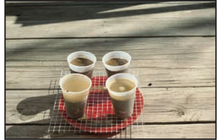
This simple test helps compare the ability of various soil types to rebound from heavy rain. Holes in the bottom let water run out, and the samples are checked to see which one firms up most quickly.
