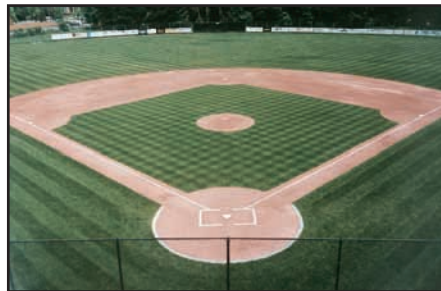
The same field, after being completely rebuilt, including the installation of PLAYBALL! ® conditioner on the skinned areas.
